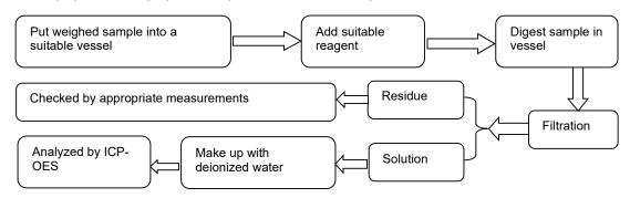
2. Test for Mercury (Hg) contents (IEC 62321-4 Ed1.0:2013):
